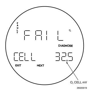
Figure 3-22. O<sub>2</sub> CELL mV
